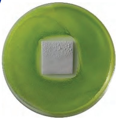
Mold test ASTM D5589 Result: No Algae growth on sample
