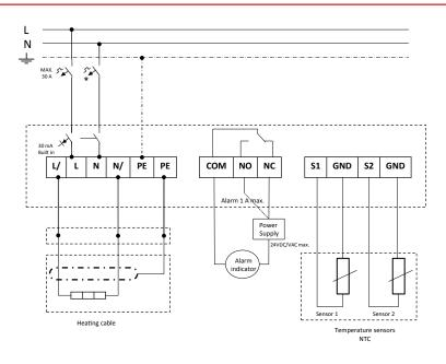
Size power supply terminals  $3 \times 6 \text{ mm}^2 \text{ maximum/10 AWG}$  Size heating cable terminals  $3 \times 6 \text{ mm}^2 \text{ maximum/10 AWG}$  Size alarm terminals  $3 \times 1,5 \text{ mm}^2 \text{ maximum/16 AWG}$  Size sensor terminal - boiler  $2 \times 1,5 \text{ mm}^2 \text{ maximum/16 AWG}$  Size sensor terminal - pipe  $2 \times 1,5 \text{ mm}^2 \text{ maximum/16 AWG}$
