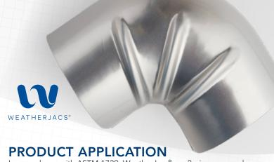
In accordance with ASTM 1729, WeatherJacs® are 2-piece pressed fittings which are pre-formed for 45 & 90 degree insulated bends conforming to ASTM, C-585 & C-450 standards. Available sizes range from ½" up through 30" NPS in long and short radius. Socket weld sizes are available from ½" through 3".
