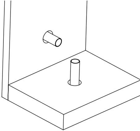
Areas to be protected must be clean and free of oil, loose dirt, rust or scale. Installation temperatures must be between 35°F (2°C) and 100°F (38°C). Allow product to dry a minimum of 24 hours before exposure to moisture. Consult appropriate manufacturer's drawing for system design requirements. Forming or packing materials are required as an integral part of various system designs.
