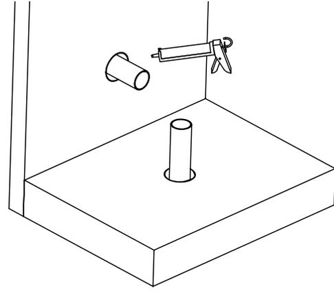
Sealant may be installed by caulking using a standard caulking gun or from bulk containers using a bulk loading caulk gun, or by manually troweling using a mason's trowel or putty knife.
