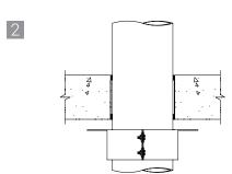
Loosely assemble collar together using provided nuts, bolts and washers at two locations on the collar flange. Insert bolt through flat washer, then through flanges in the collar, followed by a second washer and the nut.
