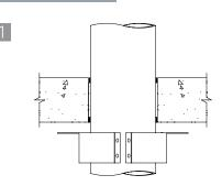
Install SpecSeal® Firestop Sealant (if required). With anchor tabs facing the mounting surface, flex collar open and wrap around pipe.
