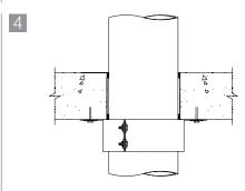
Install fasteners completely to finish collar installation.
