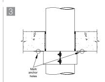
Slide collar to wall or floor surface, tighten nuts and bolts and mark anchor holes for drilling at holes in anchor tabs
