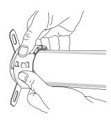
Press slots down and back (towards mounting surface) over hooks and lock into the closed position.
