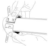
Flex collar open and wrap around pipe, anchor tabs to be facing mounting surface
