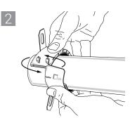
Overlap ends of collar so that the slots align over hook tabs.
