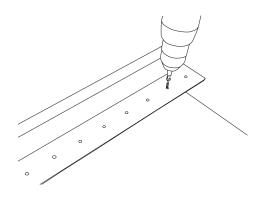
Position cut angle section so that it extends 2" (51 mm) beyond both ends of duct. Press angle in towards barrier, trapping firestop gasket between flange and barrier. Attach angle to duct using #10 x 1/2" (13 mm) steel sheet metal screws. Repeat process with bottom angle. Position screws 1" (25 mm) from each end and 6" (152 mm) center-to-center using pre drilled holes in angle.
