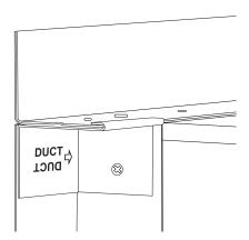
Measure and cut two vertical sections to fit tightly between the previously installed top and bottom angle sections. Corner clips are used to secure vertical and horizontal angles at all corners. Right and Left clips are provided. Clips install over vertical sections and clasp flange of extended horizontal angles. An arrow is stamped on corner clip to assist with proper orientation.
