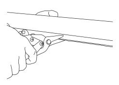
Measure and cut two sections of FyreFlange® Angle 4" (102 mm) longer than duct top and bottom width. NOTE: Tin snips or saw with metal cutting blade may be used for cutting flange. EXERCISE CARE TO AVOID DAMAGING FIRESTOP GASKET.
