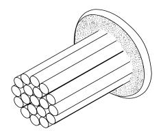
Cables to be centered within plug using slit opening. Rounded face of plug positioned outward and flush with wall surface on both sides of wall.
