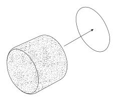
Insert plug into opening/sleeve on both sides of wall with rounded face positioned outward. Face of plug to be flush with wall surface.
