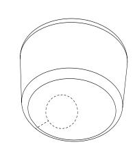
Cut hole in plug approximately the same size as the drain pipe, plug may also be slit for easier installation around drain line.
