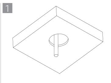
Inspect area to be protected. Remove sharp edges or protruding wires or ties that can damage foam plugs.
