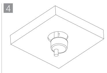
Slide plug along drain pipe into opening. Flat surface of plug to be flush with bottom surface of floor.
