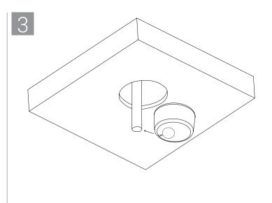
Open the plug at the slit and place it snug around drain pipe.
