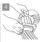
Push outer shell towards the wall, sandwiching the gasket.
