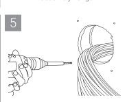
Using the hardware supplied, drill appropriate size hole and install anchors.
