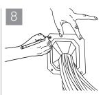
Slide inner shell towards wall (and into the outer shell from the other side), mark hole locations and slide inner shell back
