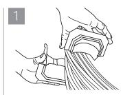
Wrap outer (larger) pathway shell assemblies around cables and align them. Attach them together completely until there are audible clicks.
