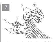
Wrap inner (smaller) pathway shell assemblies around cables and align them. Attach them together completely until there are audible clicks.
