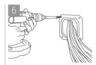
Secure outer shell to the wall using provided screws.
