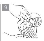
Cut gasket and wrap around inner shell assembly flange.
