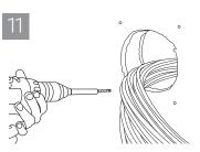
Using the hardware supplied, drill appropriate size hole and install anchors.
