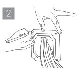
Slide outer shell towards wall, mark hole locations and slide outer shell back.
