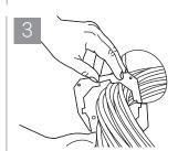
Cut gasket and wrap around outer shell assembly flange.
