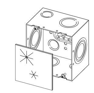
Align edge of pad to top of box and center pad. Press pad firmly against back inside wall of electrical box. Hold insert in place for 30 seconds Note: Once in place, insert is not repositionable without damaging the adhesive.
