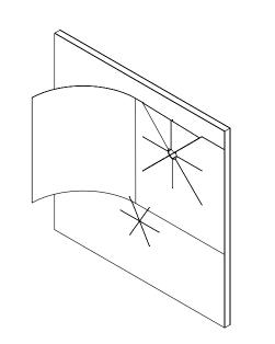
Remove protective liner from adhesive tape on back of pad.
