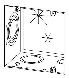
After installation of the insert, install switch or outlet.
