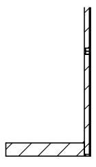
Install sealant to required depth. Work sealant into all areas exercising care to eliminate voids or seams. The surface of the sealant can be smoothed using a putty knife dipped in water. Adding water to the sealant itself is not recommended.
