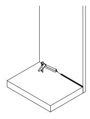
Sealant may be installed by caulking using a standard caulking gun or from bulk containers using a bulk loading caulk gun, or by manually troweling using a mason's trowel or putty knife.
