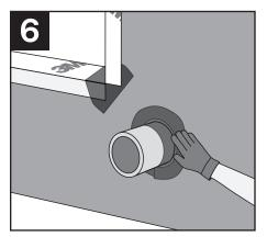
Detail penetrations by wrapping 3M<sup>™</sup> Ultra Conformable Flashing Tape 3015UC around the penetration, ensuring the lap ends at the bottom with a minimum of a 2" overlap.
