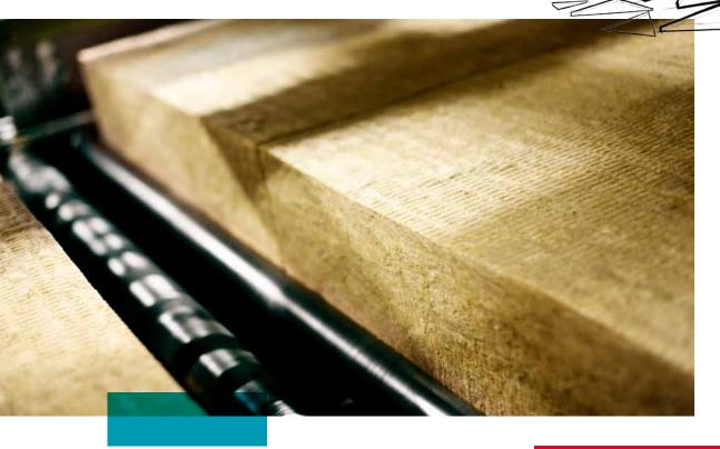
FABROCK™ Batt stone wool insulation is engineered to be fabricated and used in an OEM application. Historically used where acoustical performance and fire resistance are primary concerns, FABROCK™ Batt has excellent sound and thermal properties.
