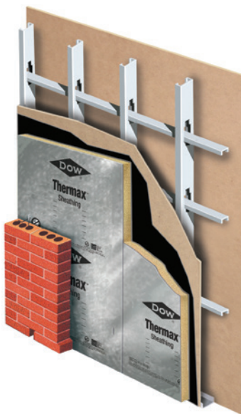
Steel Stud Hourly Rated System
