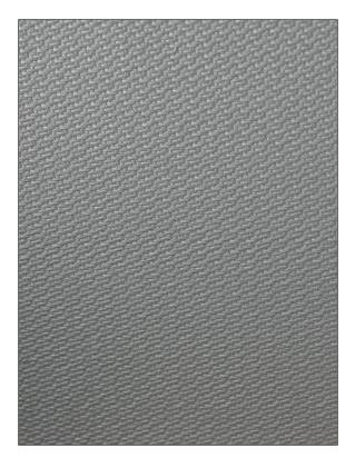
Burst Strength Method: FTMS 191A/M5122 (Mullen), 175 lbs. in. min. avg. Hydrostatic Resistance Method: FTMS191A/M5512 (Mullen), 200 lbs. in. min. avg.
