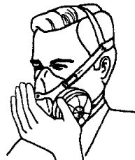
FIGURE 10: Positive Pressure Seal Check
