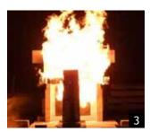
**1, 2, 3** Specialized third-party jet fire tests on FOAMGLAS® insulation in progress.
