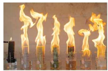
Undeniable proof of fire safety in the wicking test. Flammable liquids wick through and soak insulation materials
